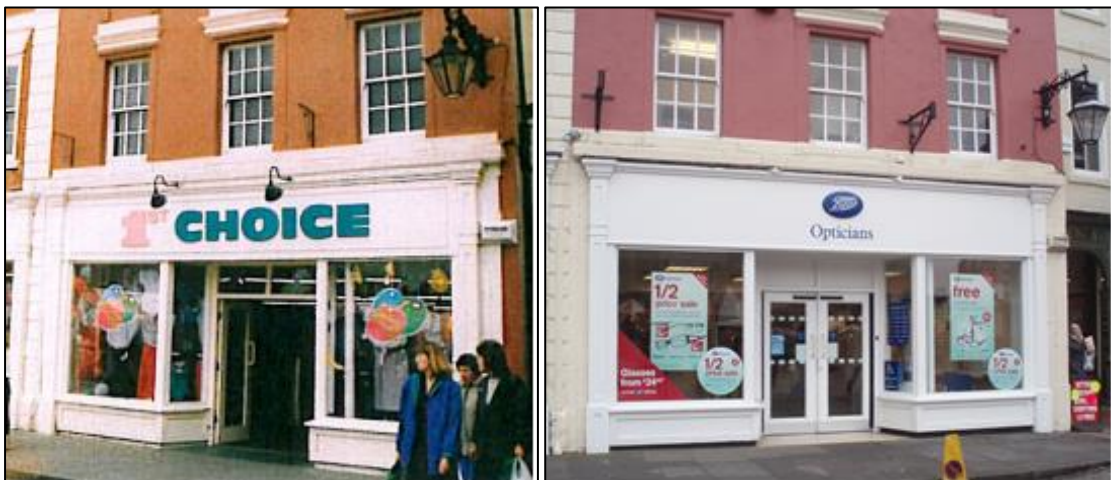
Figure 30: Removal of swan neck lighting.
