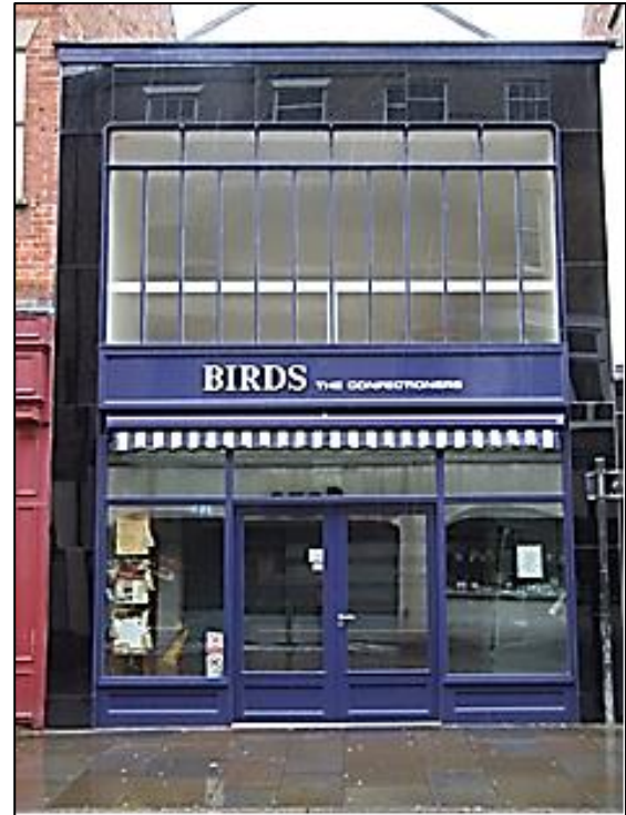
Figure 16: The poorly designed shopfront with large plate glass dating from the 1960s has been replaced with a new timber shopfront. This incorporates the elements of a traditional shopfront whilst avoiding a pastiche and compliments its wider setting within a Conservation Area.
