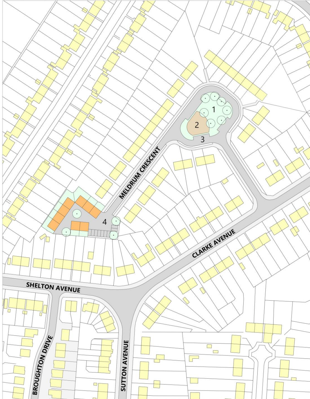
(1:1000) Proposal for regeneration of Meldrum Crescent, including elderly bungalows at existing garage court
